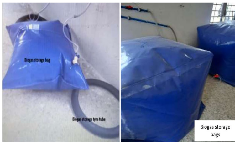
Fig. 5 A representative cross section of the different biogas storage bags used for the daily collection of the biogas generated from the mono-digestion and co-digestion of biowastes in Bayelsa State, Niger Delta, Nigeria. Black tyre tube, 2 L (left), small biogas storage bag, 500 L (left), medium biogas storage bag, 4000 L (right). The maximum pressure the bags can withstand 4 mBar
