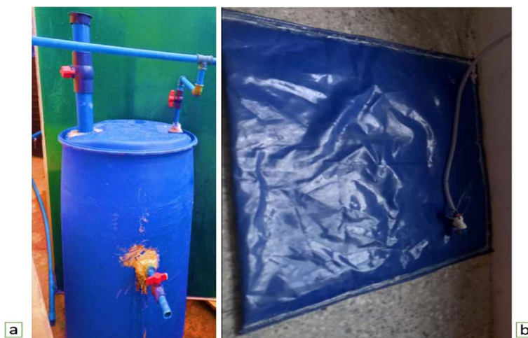
Fig. 2 a A representative biodigester set up and b A representative biogas storage bag
